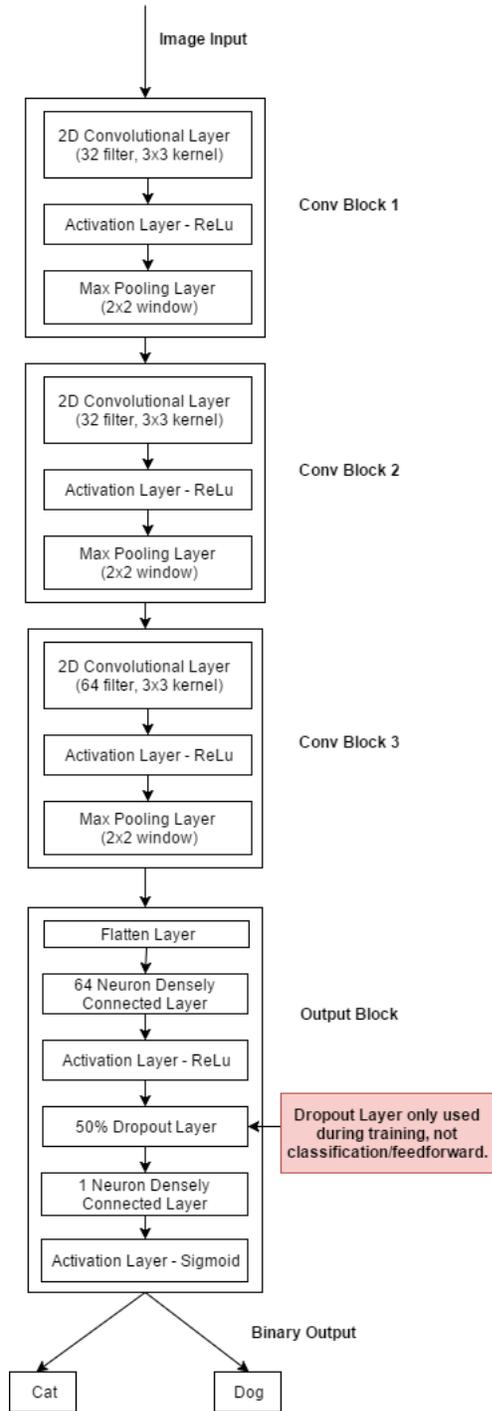
Fig. 4. Design of Neural Network using a reworked LeNet Structure
