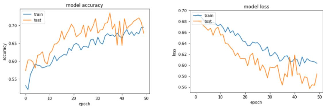
Fig. 12. Model accuracy and model loss of the CNN using filter size of 2, 2, 4, 4
