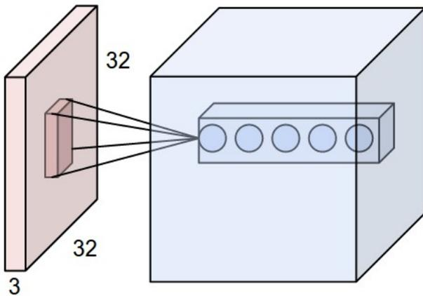
Fig. 2. An example of how convolutional layers work
