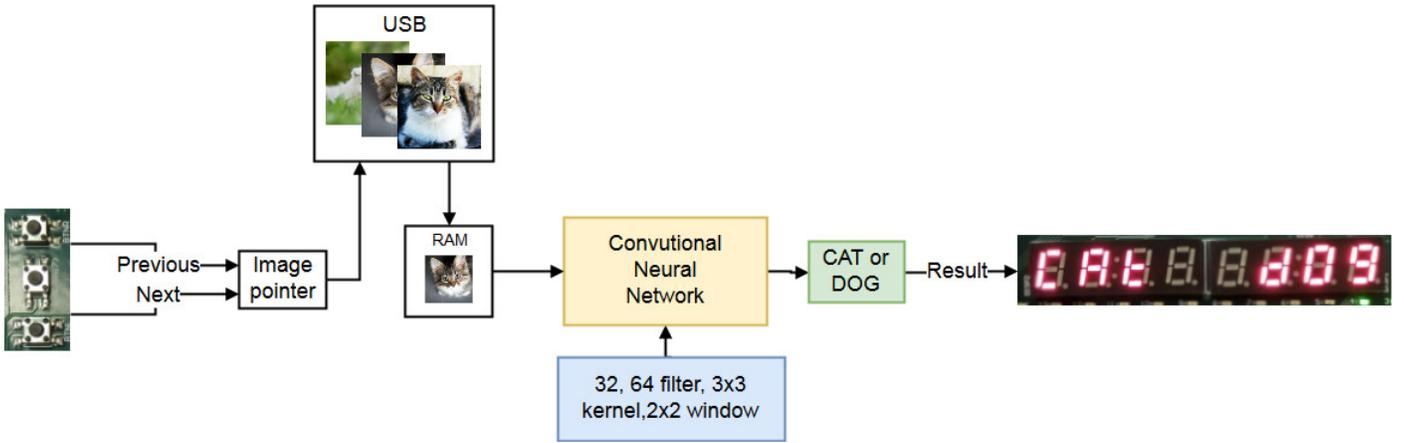
Fig. 3. Prototype design of the FANN
